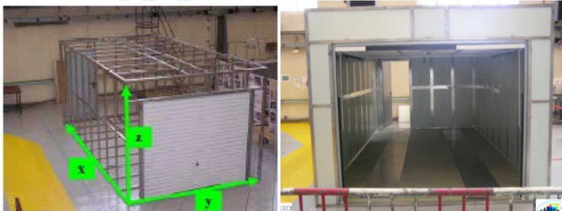
Figure 2-1. Description of GARAGE set-up at CEA Saclay. GARAGE structure showing front and service door (left) and GARAGE structure equipped with Styrodur® sheets (right).
