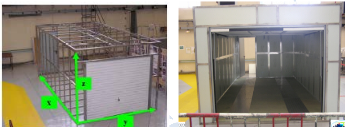
Figure 2-14. GARAGE set-up at CEA Saclay, Left: structural steel skeleton and Right: interior of the facility with the panels.
