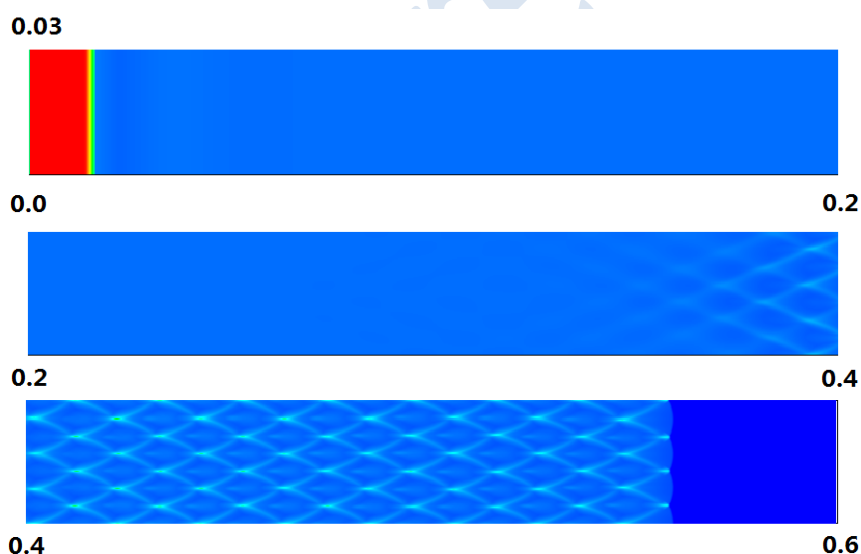
Figure 4.3-9. Numerical smoke-foil record of simulation with resolution 0.25 mm.
